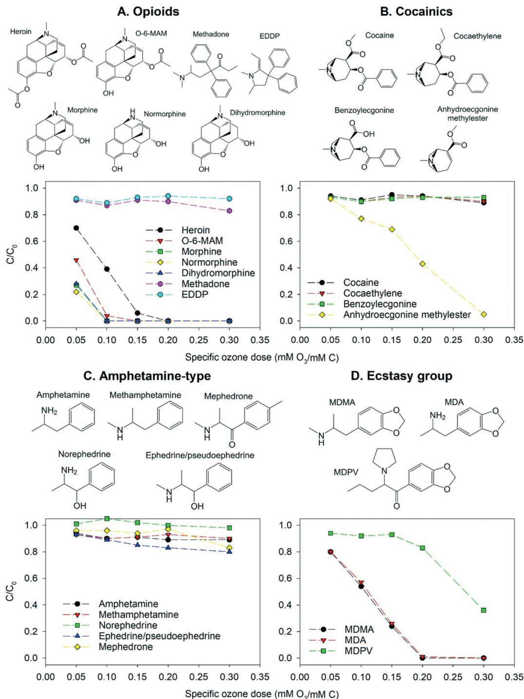
**Fig. 2** Abatement of illicit drugs and their metabolites as a function of the specific ozone dose in pure buffered water at pH 7. All compounds were added as a mixture of 90 OMPs in total. Error bars from duplicate analysis of samples were omitted for figure overview and are provided in the ESI† xlsx-data file.
