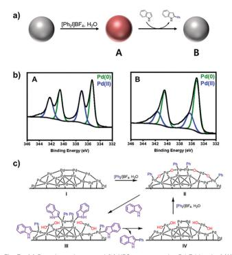
Fig. 3 (a) Reaction scheme and (b) XPS spectra at the Pd 3d level of (A) oxidized Pd NPs after the treatment with [Ph2I]BF4 and (B) after C-H arylation in air. (c) Proposed catalytic cycle.
