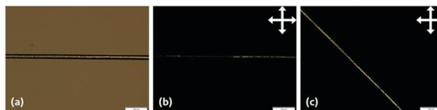
Fig. 6 A PI fibre spun from a 14% w/w PI in *n*-hexane dope with a core consisting of the liquid crystal mixture RO-TN 615. Scale bars indicate 100 μm. (a) A fibre viewed under a single polariser. (b) The same fibre in (a) viewed between crossed polarisers; arrows indicate the direction of the linear polarisers. (c) As (b), but upon 45° clockwise rotation, showing birefringence that differs from Fig. 4(b) in being of higher order.<sup>39</sup>
