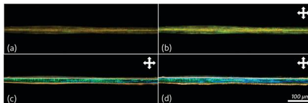
**Fig. 10** A PI fibre filled with a mixture of 25% w/w ZLI-3786 in RO-TN 615. Scale bars indicate 100  $\mu\text{m}$ . Viewed in reflective mode (a) without crossed polarisers and between crossed polarisers (b) with normally incident illumination; (c) with obliquely incident illumination from  $\sim 45^\circ$ ; (d) with obliquely incident illumination from  $\sim 60^\circ$ .
