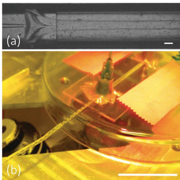
**Fig. 3** Jetting of poly-*cis*-isoprene in a bath of 10% PVP (w/w) and 7% LiBr (w/w) in ethanol without a heterocore, viewed (a) under the microscope and (b) macroscopically, with the PI fibres visible in the form of a thin, spiralling white helix exiting the spinneret device. The flow rates are 2.0 mL h<sup>-1</sup> outer phase and 0.55 mL h<sup>-1</sup> inner phase. Scale bars are 200 μm in (a) and 25 mm in (b).
