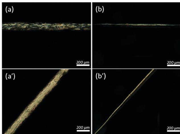
Fig. 7 Samples of thicker PI fibres spun from 14% PI in *n*-hexane dope and filled with RO-TN 615. Scale bars 200  $\mu\text{m}$ . Bottom images correspond to the upper images, with the sample rotated by 45° counterclockwise, showing a substantial brightening when the fibre no longer lies along either of the polariser axes. Both (a) and (b) represent different fibre samples without stretching.
