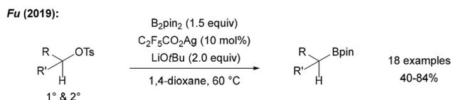
Scheme 28 Ag-mediated radical borylation of alkyl tosylates using B<sub>2</sub>pin<sub>2</sub>.
