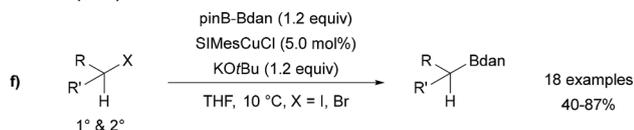
Scheme 23 Cu catalyzed borylation of alkyl halides using B<sub>2</sub>pin<sub>2</sub> (a, b, c and e), B<sub>2</sub>neop<sub>2</sub> (d) and pinB-Bdan (f).
