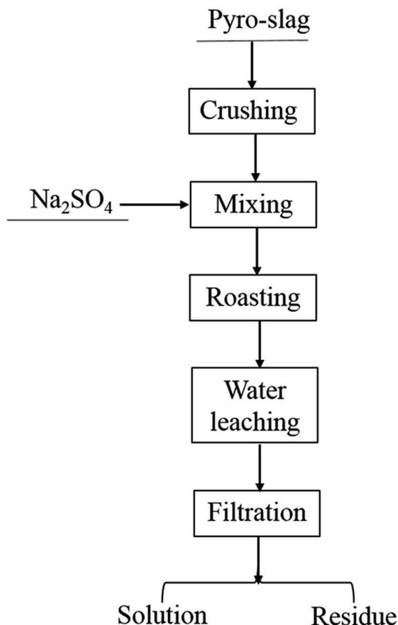
Fig. 4 Flow sheet for the roasting-leaching process.
