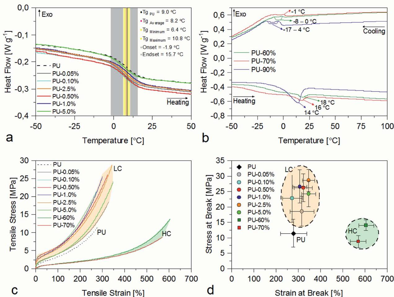
Fig. 3 (a) DSC heat flow curves for low concentration nanocomposites compositions and (b) for the highly concentrated Mag@PB<sub>1000</sub>/PU nanocomposites; (c) tensile stress–strain curves and (d) break points of the tensile test of Mag@PB<sub>1000</sub>/PU nanocomposites.
