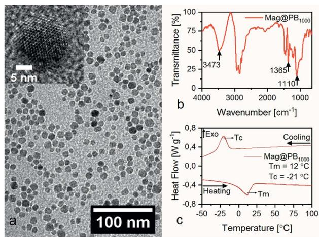
Fig. 1 (a) TEM image, the inset shows HR-TEM image of a freestanding NP. (b) FTIR analysis and (c) DSC heat flow analysis of Mag@PB<sub>1000</sub> nanoparticles.
