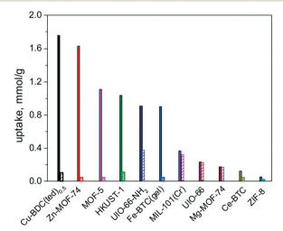
Fig. 1 H<sub>2</sub>S uptake on different MOFs at 298 K under 1 atm (H<sub>2</sub>S, 1 kPa; filled column: fresh MOF adsorbents; striped column: refreshed adsorbents). Reproduced with permission from ref. 38.
