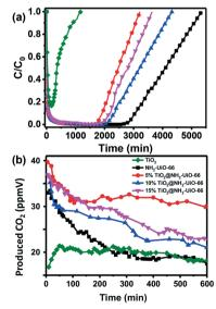
Fig. 6 Adsorption kinetic curves of styrene (a) and evolution of  $CO_2$  from photocatalytic degradation of styrene after adsorption equilibrium onto adsorbent (b) by  $TiO_2$ ,  $NH_2$ -UiO-66 and  $TiO_2@NH_2$ -UiO-66 composites. Reproduced with permission from ref. 150.
