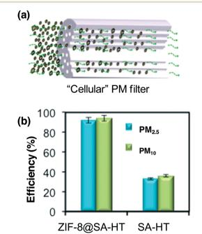
Fig. 3 (a) Schematic illustration of a "cellular" PM filter. (b) The removal efficiency of the "cellular" PM filter as well as a reference sample. Reproduced with permission from ref. 120.
