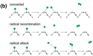
Fig. 2 The possible adsorption mechanism of halogens on MOFs (a) and the possible desorption pathways (b). Reproduced with permission from ref. 48.
