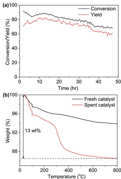
**Fig. 6** (a) Stability test for Ni/Al<sub>2</sub>O<sub>3</sub>-PD catalyst. 1-Hexanol at 1  $\mu\text{L min}^{-1}$  with 8 mL  $\text{min}^{-1}$  NH<sub>3</sub> and 20 mL  $\text{min}^{-1}$  N<sub>2</sub> flowed through 200 mg catalyst at 230 °C. GHSV =  $1.12 \times 10^4 \text{ h}^{-1}$ . (b) TG analysis for Ni/Al<sub>2</sub>O<sub>3</sub>-DP catalyst before and after reaction.
