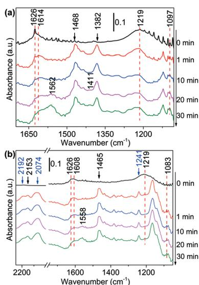
**Fig. 4** DRIFTS of adsorbed species on NH<sub>3</sub> saturated Ni/Al<sub>2</sub>O<sub>3</sub>-DP surface as a function of time under N<sub>2</sub> flow at 130 °C. At *t* = 0 min, (a) 1-butanol and (b) 1,1-dideuteriobutan-1-ol was injected.
