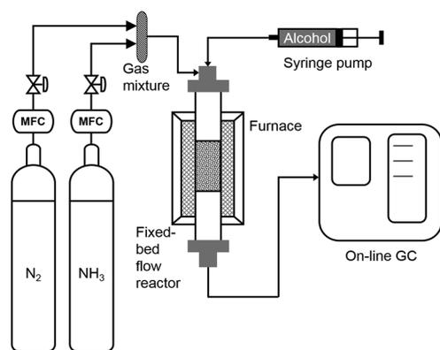
**Scheme 1** Experimental set-up for the conversion of alcohols to nitriles.
