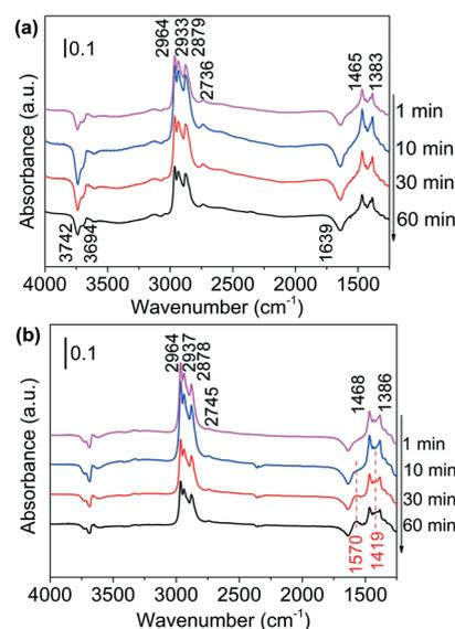
Fig. 3 DRIFTS of adsorbed species on (a)  $\text{Al}_2\text{O}_3$  surface and (b) Ni/ $\text{Al}_2\text{O}_3$ -DP surface as a function of time under  $\text{N}_2$  flow at  $130 \text{ }^\circ\text{C}$ . At  $t = 0 \text{ min}$ , 1-butanol was injected.
