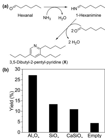
**Fig. 1** (a) Scheme for formation of 3,5-dibutyl-2-pentyl-pyridine (compound X) and (b) yield of compound X with different supports. Reaction conditions: 1 μL min<sup>-1</sup> hexanal, 200 mg catalyst, 190 °C, 8 mL min<sup>-1</sup> NH<sub>3</sub>, 20 mL min<sup>-1</sup> N<sub>2</sub>. GHSV = 1.12 × 10<sup>4</sup> h<sup>-1</sup>.
