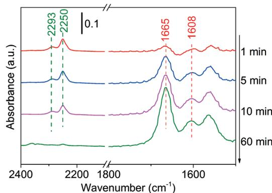
**Fig. 5** DRIFTS of adsorbed butanenitrile on Ni/Al<sub>2</sub>O<sub>3</sub>-DP surface as a function of time under N<sub>2</sub> flow at 100 °C. At *t* = 0 min, butanenitrile was injected.
