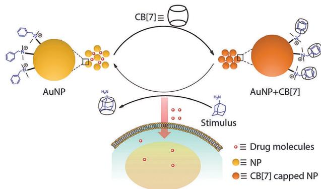
**Scheme 1** Dynamic nanoparticle assembly and design of a small molecule stimuli responsive drug delivery system. Assembly of AuNPs driven by CB[7] and disassembly by ADA due to host–guest complexation of CB[7] with ADA. Triggered release of drug molecules from assembly and uptake by the cell.
