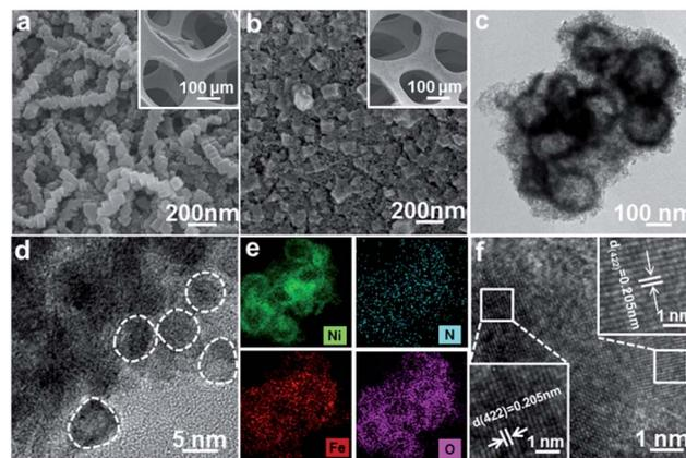
Fig. 2 SEM images of (a) initial  $\text{NiFe}^{\text{II}}$ -PBA/NF without heat treatment, (b)  $\text{NiFe}^{\text{II}}$ -PBA-SE/NF-400, (c, d, f) HRTEM images and (e) the elemental distribution mapping of  $\text{NiFe}^{\text{II}}$ -PBA-SE/NF-400.
