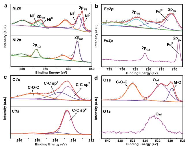
Fig. 3 XPS spectra of (a) Ni 2p, (b) Fe 2p, (c) C 1s and (d) O 1s for initial NiFe<sup>II</sup>-PBA and NiFe<sup>II</sup>-PBA-SE/NF-400 (with the bottom spectra corresponding to initial NiFe<sup>II</sup>-PBA without heat treatment and the upper spectra corresponding to NiFe<sup>II</sup>-PBA-SE/NF-400).
