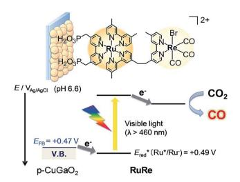
Scheme 16 Schematic illustration for the photocatalytic reduction of  $CO_2$  to CO with the  $RuRe/CuGaO_2$  electrode. Reprinted with permission from ref. 173. Copyright 2017, Royal Society of Chemistry.
