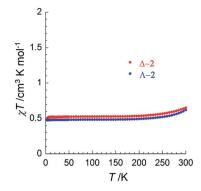
Fig. 3 Temperature dependence of the  $\chi T$  product for  $\Delta$ -2 (red) and  $\Lambda$ -2 (blue) at 0.1 T, where  $\chi$  is the magnetic susceptibility defined as M/H per mole of complex, with M being the magnetization and H the applied magnetic field.
