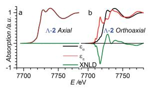
Fig. 4 XANES and XNLD spectra obtained with linearly polarized X-rays for (a) axial ( $\theta = 0^{\circ}$ ) and (b) orthoaxial ( $\theta = 90^{\circ}$ ) configurations.
