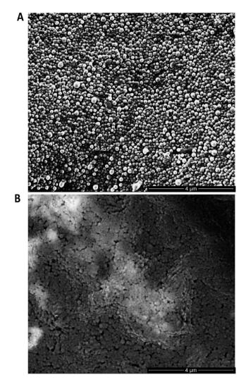
Fig. 3 ESEM imaging of nanoformulations. (A) Modified TRAZ F(ab) NP [disulfide] and (B) native TRAZ F(ab) NP were dried on double-sided copper tape mounted onto aluminium stubs, sputter-coated with gold and imaged with an ESEM. Scale bar  $=4~\mu m$ .
