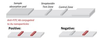
Fig. 2 Illustrative representation of the principle of the lateral flow test strips employed.
