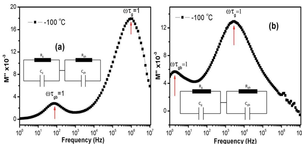
Fig. 11 The  $M''$  vs. frequency behaviour for LCO and Ir doped LCO just at  $-100\text{ }^\circ\text{C}$  and the relaxation points ( $\omega_{\max}\tau = 1$ ). Inset figures show equivalent circuit for each compounds.
