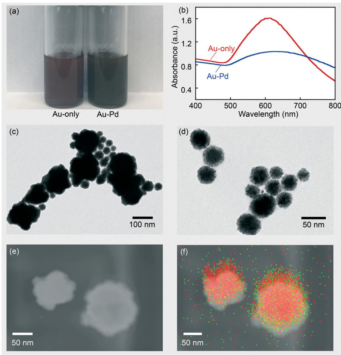
**Fig. 5** (a) Au and Au-Pd nanoparticle re-dispersed in deionized water. (b) UV-vis spectrum of Au nanoparticles and Au-Pd core-shell nanoparticles. (c) and (d) TEM images of the prepared Au-Pd core-shell nanoparticles. (e) and (f) TEM-EDS characterization of the large nanoparticles ( $\sim 100$  nm) with red signal from gold and green signal from palladium atoms.
