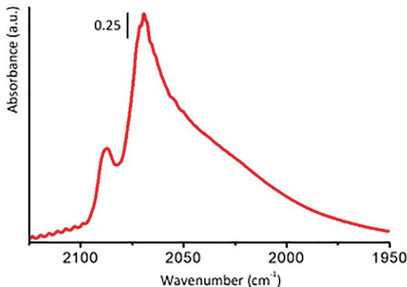
Fig. 7 FT-IR spectrum of CO adsorbed at room temperature on a 5 wt% Pt/Al<sub>2</sub>O<sub>3</sub> catalyst similar to the Pt/C investigated in this work.
