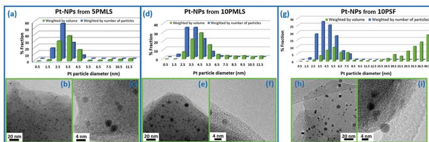
Fig. 3 Particle size distribution weighted by number (blue, from a TEM study) and by volume (green, to be used to estimate the average coordination number  $N$  obtained by the EXAFS first shell analysis) in three different examples of Pt NPs formed inside a Pt-functionalized UiO-67 MOF. Adapted by permission of the Royal Society of Chemistry (copyright 2017).<sup>5</sup>
