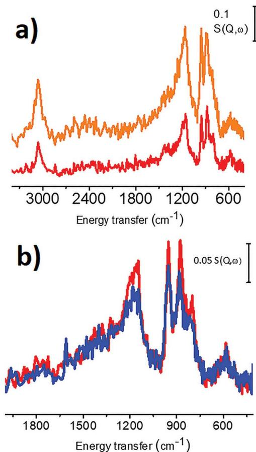
Fig. 5 Part (a) INS spectra of  $C_w$  (red spectrum) and  $C_{\text{chemi}}$  (orange spectrum). Part (b) INS spectra of  $C_w$  (red) and of the corresponding  $\text{Pd}/C_w$  catalyst (blue). Previously unpublished figure, reporting data published in ref. 1.
