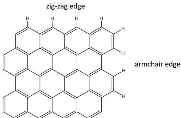
Fig. 6 Armchair termination of a graphitic sheet.
