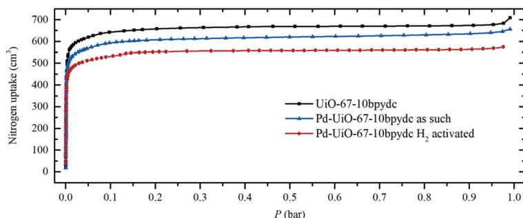
Fig. 11 N<sub>2</sub> adsorption isotherms of UiO-67 with 10% of modified ligands non-functionalized (black squares) and functionalized by Pd before (blue triangles) and after (red circles) activation in H<sub>2</sub> at 300 °C.
