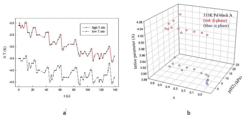
Fig. 1 (a) Exothermic synchronised oscillations seen by IRT over macroscopic distances (cm) when *Penicillium* grows on a moist, naturally-colonised surface (multigrain bread). (b) Plots of  $p_{\text{H}_2}$ - $x$  in PdH<sub>x</sub>-fcc lattice parameter at 333 K for 86 nm unsupported Pd black (where the  $\Delta x$  width of the hysteresis loop was larger than for a 10 nm sample).<sup>5</sup>
