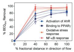
Fig. 3 Removal of BEQ<sub>bio</sub> (%) along the flow path in HM for assays indicative of activation of AhR, binding to PPARy, activation of ER, oxidative stress response and NF-κB response (eqn (3)). Samples collected in July indicated by closed symbols and solid lines; samples collected in November indicated by open symbols and dashed lines. Error bars were calculated using error propagation.
