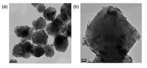
Fig. 1 (a) and (b) HR-TEM images of fresh Pd-Pt-Fe<sub>3</sub>O<sub>4</sub> NPs.
