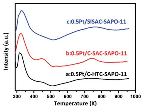
Fig. 7  $H_2$ -TPR profiles of (a) C-HTC-SAPO-11, (b) C-SAC-SAPO-11 and (c) SISAC-SAPO-11.
