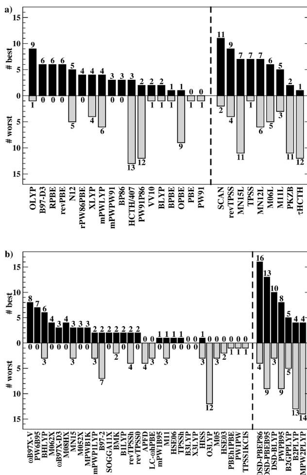
**Fig. 6** Analysis of how many times a DFA yields the worst and best MAD for GMTKN55. All DFAs were dispersion corrected, but the suffix "D3" was omitted from the labels for better clarity, unless it is needed to avoid ambiguity. The analysis was carried out separately for each of the four highest rungs on Jacob's Ladder: GGA/NGA (a, left), meta-GGA/NGA (a, right), hybrid (b, left), and double hybrid (b, right).
