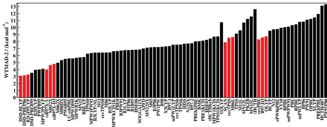
Fig. 8 Final WTMAD-2 values over the entire GMTKN55 for all assessed 83 dispersion-corrected DFAs ( $\text{kcal mol}^{-1}$ ). The red bars indicate the three best approaches on their respective rung of Jacob's Ladder. The suffix "D3" was omitted in all cases, unless it is needed to avoid ambiguity.
