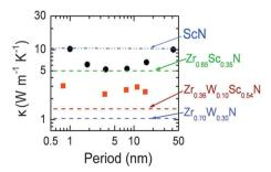
Fig. 4 Illustration of superlattice reduction in thermal conductivity, from Rawat et al.<sup>44</sup> Cross-plane thermal conductivity of 300 nm thick ZrN/ScN (dots) and Zr<sub>0.64</sub>W<sub>0.36</sub>N/ScN (squares) multilayers. Superimposed on the plot are horizontal lines corresponding to the experimentally determined lattice component of thermal conductivity, i.e., the alloy limit of different alloys of ZrN, ScN, and W2N. (Copyright American Institute of Physics, used
