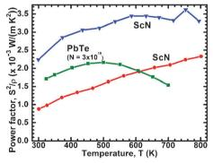
Fig. 2 Thermoelectric power factor  $S^2\sigma$  of ScN (the bottom curve shows our first data from ref. 2 and the top curve are the data of Burmistrova et al.).3 The example data for PbTe are adapted from Sootsman et al. 43
