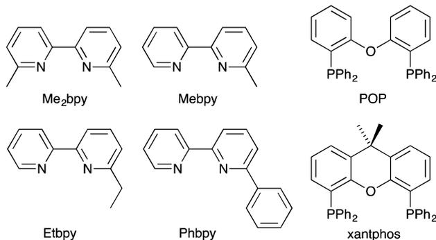
**Scheme 1** Structures of  $\text{N}^{\wedge}\text{N}$  ligands 6,6'-dimethyl-2,2'-bipyridine ( $\text{Me}_2\text{bpy}$ ), 6-methyl-2,2'-bipyridine ( $\text{Mebpy}$ ), 6-ethyl-2,2'-bipyridine ( $\text{Etbpy}$ ) and 6-phenyl-2,2'-bipyridine ( $\text{Phbpy}$ ), and the  $\text{P}^{\wedge}\text{P}$  ligands POP and xantphos.
