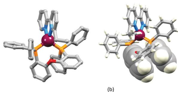
Fig. 5 Structure of the  $[\text{Cu}(\text{POP})(\text{Etbpy})]^+$  cation in  $[\text{Cu}(\text{POP})(\text{Etbpy})][\text{PF}_6] \cdot \text{Et}_2\text{O}$ : (a) view of the cation (H atoms omitted for clarity); (b) intra-cation face-to-face  $\pi$ -stacking interaction.
