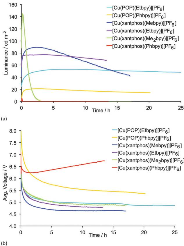
Fig. 10 Luminance (a) and average voltage (b) for ITO/PEDOT:PSS/[Cu(P<sup>A</sup>P)(N<sup>A</sup>N)][PF<sub>6</sub>] : [Emim][PF<sub>6</sub>] 4 : 1 molar ratio/Al LECs measured using a pulsed current driving (average current density 50 A m<sup>-2</sup>, 1 kHz, 50% duty cycle, block wave). [Emim][PF<sub>6</sub>] = 1-ethyl-3-methylimidazolium hexafluoridophosphate.
