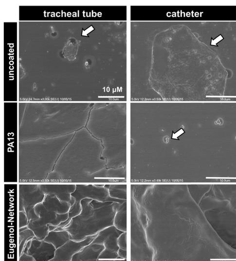
**Fig. 7** SEM images of uncoated and PA13 and Eugenol-Network coated endotracheal tube and catheter after incubation with a cocktail of *K. pneumoniae* and MRSA (scale bar 10  $\mu$ m). The arrows show surface attached bacteria.
