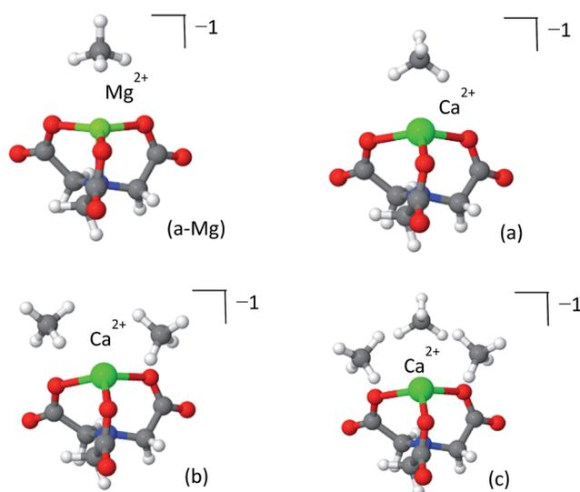
**Fig. 11** Clusters of NTA-Mg (panel a-Mg) and NTA-Ca (panels a–c) with CH<sub>4</sub>. The first adsorbed CH<sub>4</sub> NTA-Mg blocks the adsorption site, while three CH<sub>4</sub> can adsorb to the pyramidal NTA-Ca.
