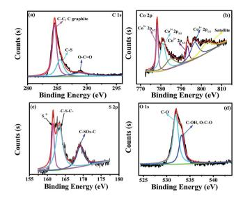
Fig. 3 High-resolution C 1s XPS spectra (a), Co 2p spectra (b), S 2p spectra (c) and O 1s spectra (d) of the as-obtained  $Co_3S_4-S/G-800$  hybrids.
