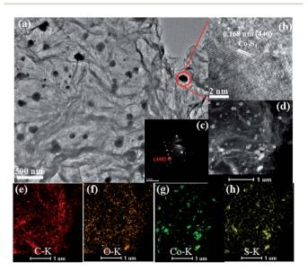
Fig. 2 TEM images (a), HRTEM image (b), SAED pattern (c), HAADF-STEM (d) and elemental mapping images (e-h) of  $Co_3S_4$ -S/G-800 catalyst.
