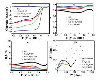
Fig. 5 LSV curves (a) electron transfer number (b) and  $H_2O_2$  yield (c) of S/G,  $Co_3S_4/C-800$ , S/G +  $Co_3S_4/C-800$  (physical mixture) and  $Co_3S_4-S/G-800$  catalysts in an  $O_2$ -saturated 0.1 M KOH electrolyte with a scan rate of 5 mV s<sup>-1</sup>. EIS (d) of S/G,  $Co_3S_4/C-800$ , S/G +  $Co_3S_4/C-800$  and  $Co_3S_4-S/G-800$  modified working electrode in a solution of 5.0 mM Fe(CN) $_6$ <sup>3-/4-</sup> containing 100 mM KCl.
