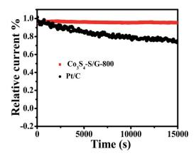
Fig. 6 Amperometric i-t curves of Co<sub>3</sub>S<sub>4</sub>-S/G-800 and Pt/C in O<sub>2</sub>-saturated 0.1 M KOH electrolyte.
