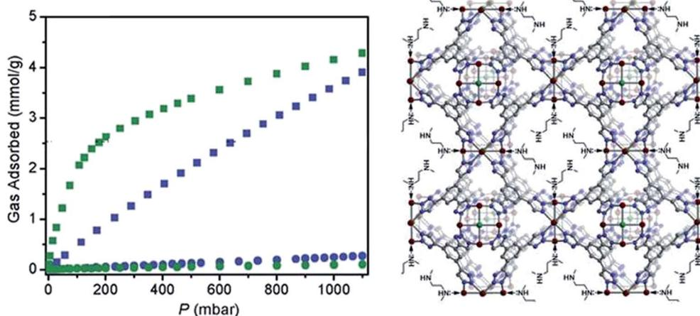
Fig. 8 Isotherms for CO<sub>2</sub> (squares) and N<sub>2</sub> (circles) adsorption at 25 °C for mmen-CuBTtri (green) and CuBTtri (blue). Reprinted from ref. 58 with permission from Royal Society of Chemistry.
