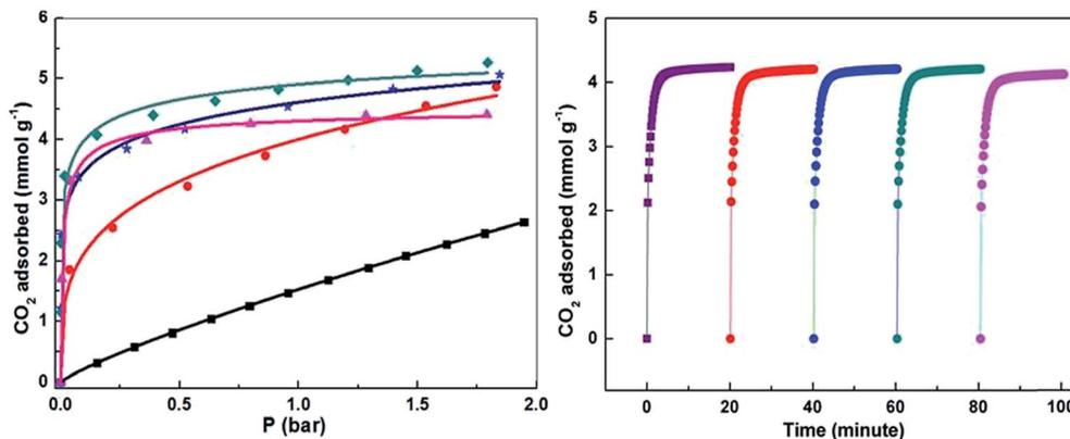
Fig. 9 (Left)  $\text{CO}_2$  adsorption isotherms of MIL-101(Cr) before and after PEI loading at  $25^\circ\text{C}$ . Symbol: ■ MIL-101, ● PEI-MIL-101-50, ★ PEI-MIL-101-75, ◆ PEI-MIL-101-100 and ▲ PEI-MIL-101-125. (Right) Cycling  $\text{CO}_2$  adsorption kinetics of PEI-MIL-101-100. Reproduced from ref. 62 with permission of Nature Publishing Group.
