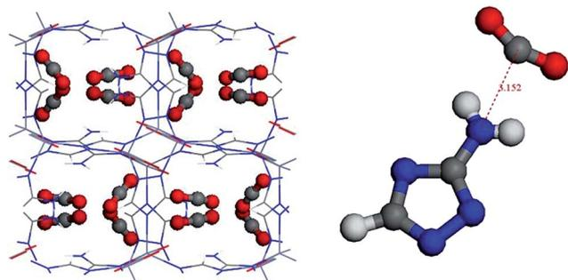
Fig. 6 Locations of CO<sub>2</sub> adsorbed in the Zn<sub>2</sub>(Atz)<sub>2</sub>. Ball: blue, N; white, H; gray, C.
