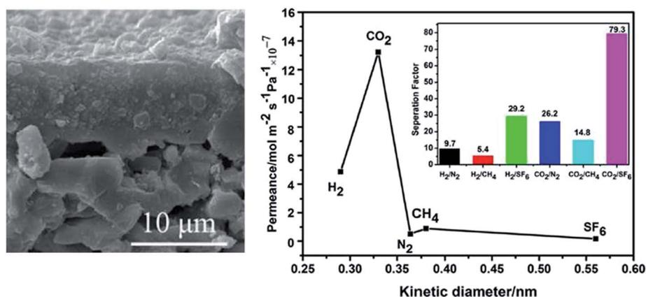
Fig. 12 CAU-1 membrane SEM image and single gas permeances at room temperature. Reprinted from ref. 84 with permission from Royal Society of Chemistry.
