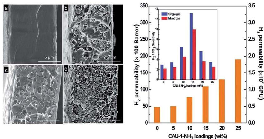
Fig. 14 Left: SEM images of the cross section of pure poly(methyl methacrylate) membrane (a) and MMMs with 5 wt% (b), 15 wt% (c) and 25 wt% (d) CAU-1 loading. Right: H<sub>2</sub> permeability of the MMMs with different CAU-1 loadings and the corresponding H<sub>2</sub>/CO<sub>2</sub> selectivities (inset). Reprinted from ref. 95 with permission from Royal Society of Chemistry.
