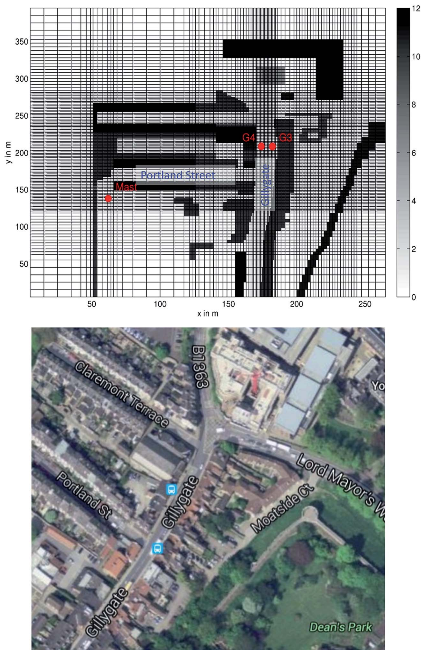
Fig. 1 Top: Site schematic for the York Gillygate site showing the grid and building configuration as used in MISKAM. Bottom: Aerial view of the site. ©2015 Infoterra Ltd. & Bluesky, ©2015 Google.
