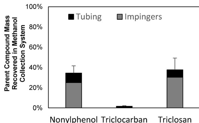
Fig. 4 The impact of pyrolysis on the fate of microconstituents spiked into sand. No microconstituents were detected in sand following pyrolysis at 500 °C for two hours. Following pyrolysis the mass recovered in the methanol collection system (tubing + impingers) was highest for NP and TCS which had the highest vapor pressures. The error bars represent the standard deviation observed among the total amounts of mass recovered for each microconstituent between the triplicate runs ( $n = 3$ ).
