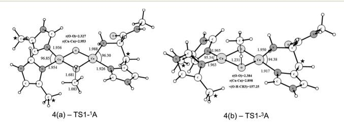
Fig. 5 Optimized structures of the transition states (singlet and triplet) involved in the C-H bond activation step. Bond length and angles are given in Angstrom and degrees, respectively. The coordinates of the atoms highlighted with a star were kept fixed during the geometry optimization.
