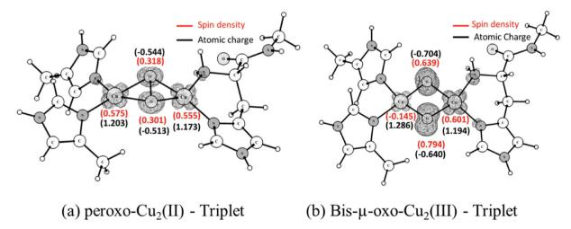
Fig. 4 Calculated Mulliken spin densities and atomic charges for the triplet state of peroxo- $Cu(III)_2$  and  $bis(\mu-oxo)Cu(IIII)_2$  complexes. Spin densities are shown in red and atomic charges in black.
