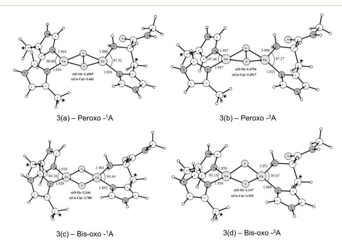
Fig. 3 B3LYP-D2/BSI optimized structures of the singlet and triplet states of the peroxo and bis-µ-oxo intermediates generated from the interactions of the O<sub>2</sub> molecule with the binuclear copper center of pMMO. Bond length and angles are given in Angstrom and degrees, respectively. The coordinates of the atoms highlighted with a star were kept fixed during the geometry optimization.
