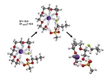
Fig. 7 Calculated structures of pre-reaction complexes, transition states and post-reaction complexes in the mechanism for the reaction  $[K^+F^- + C_3H_7 - OMs \rightarrow K^+OMs^- + C_3H_7 - F]$  in tetraEG. Energy and Gibbs free energy in kcal  $\text{mol}^{-1}$  and bond lengths in Å (MPW1K/6-31++G\*\*).
