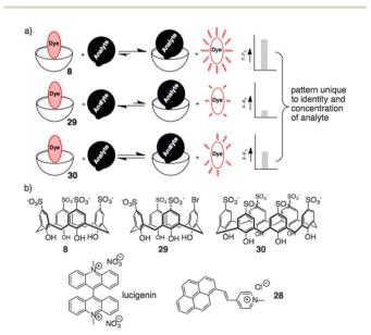
Fig. 13 (a) Schematic representation of a chemical sensor array based on indicator displacement. (b) Sensor array components: calixarenes 8, 29, and 30 were combined with either lucigenin or dye 28 to create threeelement sensor arrays for analysis of post-translationally modified amino acids and peptides
