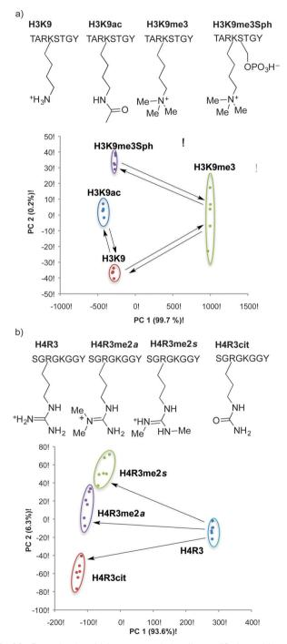
Fig. 14 Examples in which post-translationally modified peptides are identified by a simple, three-calixarene sensor array after principle component analysis. Arrows indicate peptides that are related to each other as the starting materials and products of known enzymatic transformations.
