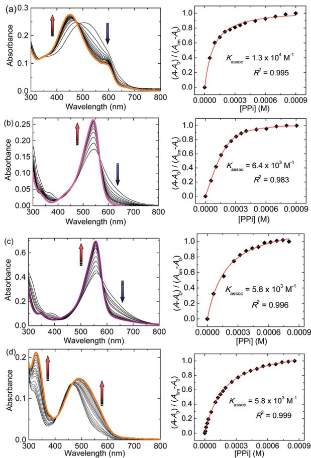
Fig. 4 UV-vis spectra of the 1-Zn-dye complex upon the addition of PPI in HEPES buffer (10 mM) with sodium chloride (10 mM) at 7.5 at 25 °C. [1-Zn] =  $6.0 \times 10^{-5}$  M. [Dye] =  $2.0 \times 10^{-5}$  M. (a) PV, (b) PR, (c) BPR and (d) ARS.
