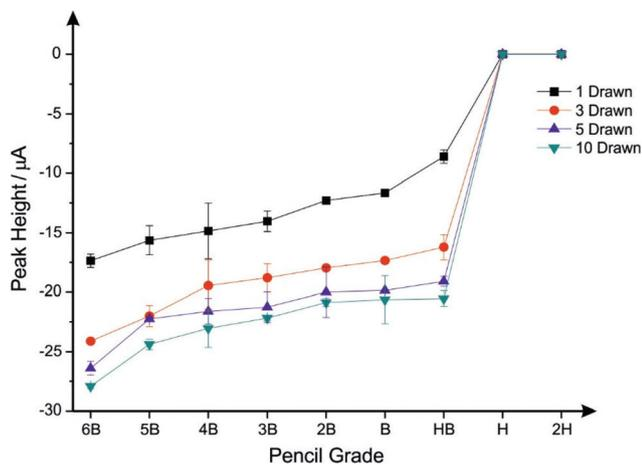
Fig. 3 Plots of pencil composition/grade vs. peak height (cathodic current) recorded in 1 mM hexammineruthenium(III) chloride/0.1 M KCl as a result of increasing the number of draws. Scan rate:  $50 \text{ mV s}^{-1}$  (vs. SCE). Data shown is an average and corresponding standard deviation ( $N = 3$ ).
