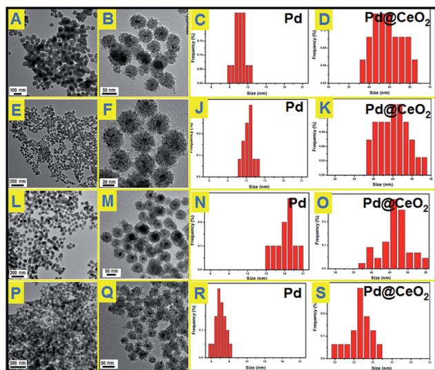
Fig. 2 TEM images and particle size distributions of Pd@CeO<sub>2</sub> core@shell nanospheres obtained by addition of different amounts of KBr in the reaction solution: (A), (B), (C) and (D) 150 mg KBr, 50  $\mu$ L NH<sub>3</sub>·H<sub>2</sub>O; (E), (F), (J) and (K) 300 mg KBr, 50  $\mu$ L NH<sub>3</sub>·H<sub>2</sub>O; (L), (M), (N) and (O) 500 mg KBr, 50  $\mu$ L NH<sub>3</sub>·H<sub>2</sub>O; (P), (Q), (R) and (S) 300 mg KBr, 200  $\mu$ L NH<sub>3</sub>·H<sub>2</sub>O.
