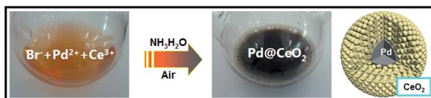
Scheme 1 The synthetic process of Pd@CeO<sub>2</sub> core@shell nanospheres.
