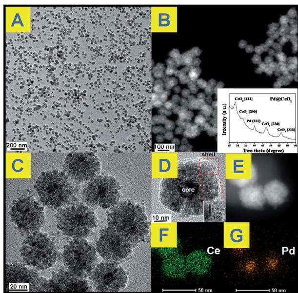
Fig. 1 (A), (C) and (D): TEM images; (B) inside; (B) and (E) STEM image; (F) and (G) mapping analysis of the as-obtained Pd@CeO<sub>2</sub> core@shell nanospheres.
