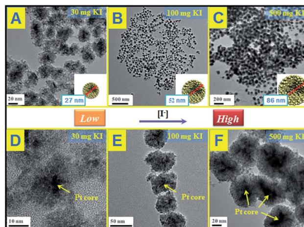
Fig. 3 TEM images of Pt@CeO<sub>2</sub> multi-core@shell nanospheres prepared by KI assistance; (A) and (D): 30 mg; (B) and (E): 100 mg; (C) and (F): 500 mg.
