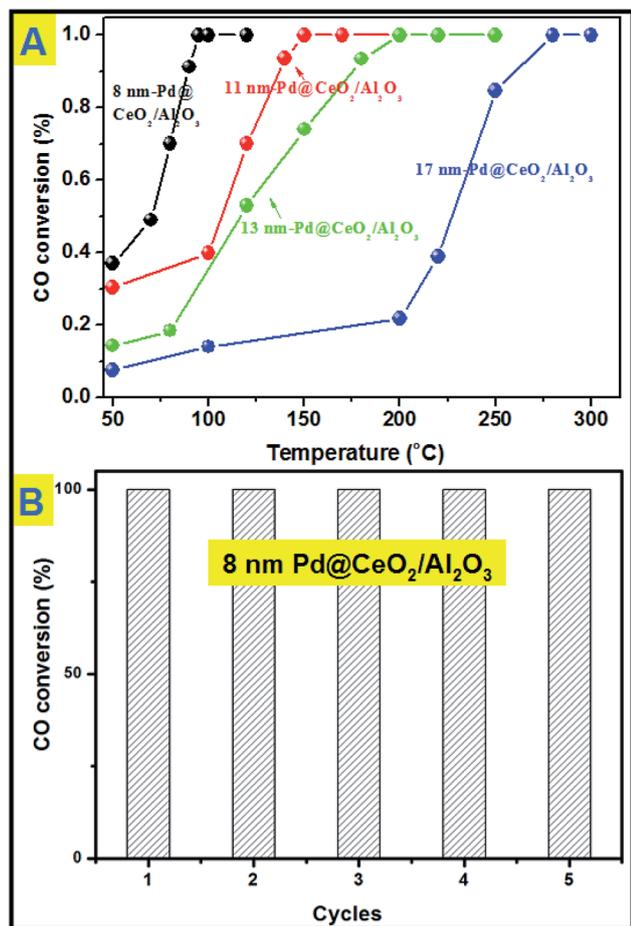
Fig. 6 (A) catalytic CO conversion of Pd@CeO<sub>2</sub>/Al<sub>2</sub>O<sub>3</sub> with different Pd core sizes; (B) cycling test of 8 nm-Pd@CeO<sub>2</sub>/Al<sub>2</sub>O<sub>3</sub>.
