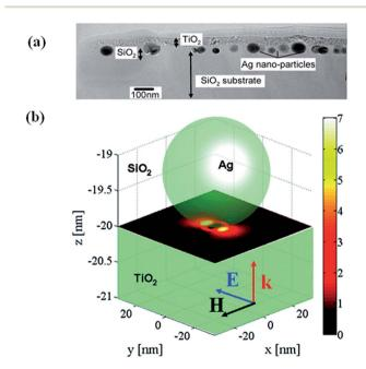
Fig. 4 (a) TEM cross sectional view showing  $TiO_2$  film on  $Ag/SiO_2$  core—shell on a  $SiO_2$  substrate. (b) Simulation showing the near-field amplitude enhancement inside a  $TiO_2$  substrate at the interface to a  $SiO_2$  substrate where a Ag NP is embedded. The y-polarized illuminating plane wave propagates in the z-direction. Reprinted with permission from ref. 56.
