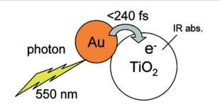
Fig. 3 Schematic representation of a gold nano dot attached on a  $TiO_2$  nanoparticle, also indicating hot electron transfer process upon the excitation of LSPR. Figure reprinted with permission from ref. 59.
