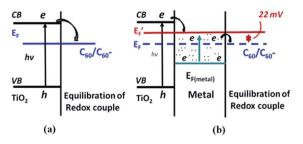
Fig. 2 Charge distribution between  $TiO_2$  and gold nanoparticles leading to equilibration with the  $C_{60}/C_{60}^-$  redox couple (a) in the absence and (b) in the presence of metal nanoparticles.  $E_F$  and  $E_F'$  refer to the Fermi levels of  $TiO_2$  before and after attaining equilibrium, respectively. Figure reprinted with permission from ref. 50.
