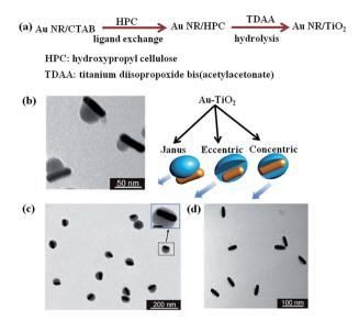
Fig. 6 (a) Preparation scheme and (b-d) TEM images of TiO<sub>2</sub>-coated gold nanorods with (b) Janus, (c) eccentric, and (d) concentric geometries. Figure reprinted with permission from ref. 77.
