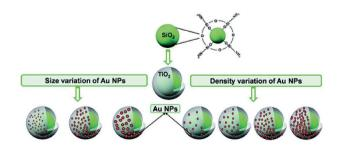
Fig. 5 Schematic illustration of the preparation protocol of core-shell SiO<sub>2</sub>/TiO<sub>2</sub> nanostructures (silica bead coated with a thin layer TiO<sub>2</sub> of 15-20 nm in thickness) and the decoration of the SiO<sub>2</sub>/TiO<sub>2</sub> surface with Au NPs. Figure reprinted with permission from ref. 70.
