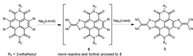
**Scheme 2** Proposed reaction process of  $\text{Na}_2(\text{i-mnt})$  with TBNDI.
