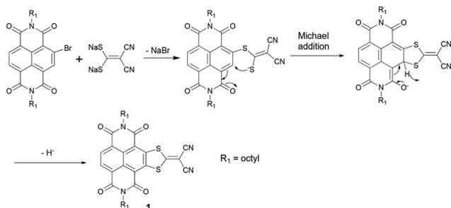
**Scheme 3** Proposed reaction mechanism of Na<sub>2</sub>(i-mnt) with monobromo NDI.
