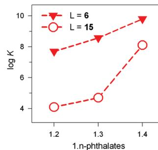
Fig. 27  $\log K$  values for the equilibria:  $[\text{Cu}^{\text{II}}_2(\text{L})]^{4+} + \text{A}^{2-} \rightleftharpoons [\text{Cu}^{\text{II}}_2(\text{L})(\text{A})]^{2+}$ , where  $\text{A}^{2-}$  is a 1, $n$ -phthalate: (i) filled triangles,  $\text{L} = 6$ , 50/50 (v/v) H<sub>2</sub>O–EtOH, 25 °C;<sup>39</sup> (ii) empty circles,  $\text{L} = 15$ , water, 25 °C.<sup>40</sup>
