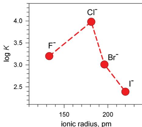
**Fig. 12** Selectivity pattern for the affinity of halides towards the dime-tallic cryptate receptor  $[\text{Cu}^{\text{II}}_2(\mathbf{3})]^{4+}$ . Log  $K$  values refer to the equilibrium:  $[\text{Cu}^{\text{II}}_2(\mathbf{3})]^{4+} + \text{X}^- \rightleftharpoons [\text{Cu}^{\text{II}}_2(\mathbf{3})(\text{X})]^{3+}$  at pH = 5.25; ( $\text{X}^-$  = halide anion).<sup>20</sup>
