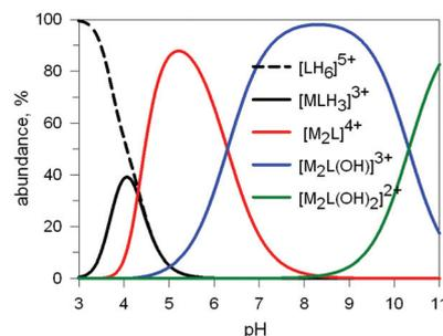
Fig. 9 Concentration (%) with respect to  $L = \mathbf{10}$  of the species present at the equilibrium for the system  $\mathbf{10}/\text{Cu}^{\text{II}}$  (ligand-to-metal ratio 1:2), in an aqueous solution 0.1 M in  $\text{NaClO}_4$ , at 25°.  $\log K$  values were obtained through a potentiometric titration.<sup>20</sup>
