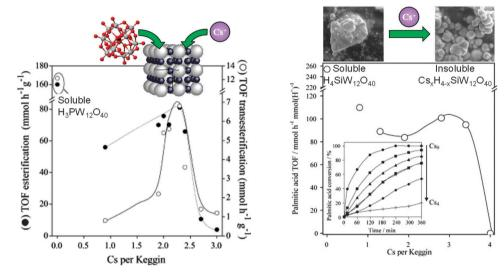
Fig. 10 Impact of Cs ion-exchange into (left) both  $Cs_xH_{(3-x)}PW_{12}O_{40}$  for palmitic acid esterification and tributyrin transesterification with methanol; and (right) and  $Cs_yH_{(y-x)}SiW_{12}O_{40}$  for palmitic acid esterification, benchmarked against parent fully protonated, soluble clusters. Adapted from ref. 138 and 177. Copyright (2007 and 2009), with permission from Elsevier.
