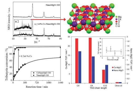
Fig. 2 Formation of crystalline  $Cs_2Mg(CO_3)_2(H_2O)_4$  phase within co-precipitated Cs-doped MgO and resulting synergy in the transesterification of short and long chain TAGs with methanol compared with undoped nanocrystalline MgO. Adapted from ref. 85 with kind permission from Springer Science and Business Media and ref. 92 with permission from John Wiley and Sons.
