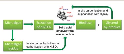
Fig. 14 Microalgae as a source of bio-oils/fatty acids for biodiesel production, and waste, biomass residue for the synthesis of solid acid catalysts to drive such biodiesel production
