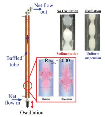
Fig. 18 Schematic of reactor flow and mixing characteristics within an OBR, and associated optical images of a PrSO<sub>z</sub>H-SBA-15 solid acid powder without oscillation (undergoing sedimentation) or with a 4.5 Hz oscillation (entrained within baffles). Adapted from ref. 42 with permission from The Royal Society of Chemistry
