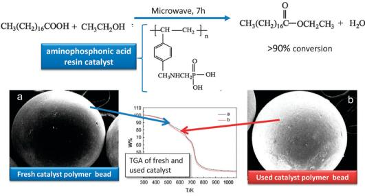
Fig. 12 Stability of a solid acid resin catalyst for stearic acid esterification. Adapted from ref. 181. Copyright (2013), with permission from Elsevier.
