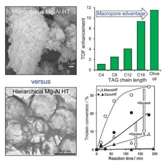
Fig. 6 Superior catalytic performance of a hierarchical macroporousmicroporous Mg-Al hydrotalcite solid base catalyst for TAG transesterification to biodiesel versus a conventional microporous analogue. Adapted from ref. 128 with permission from The Royal Society of Chemistry.
