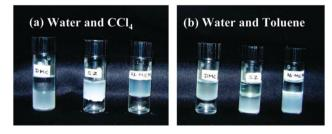
Fig. 17 Preferential dispersion of DMC in the nonpolar, organic phase, and SZ and Al-MCM-41 in the polar aqueous phase of (a) water– $CCl_4$  and (b) water-toluene solvent mixtures. Reprinted with permission from ref. 202. Copyright 2010 American Chemical Society.
