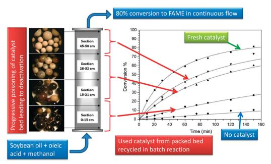
Fig. 13 Deactivation of an acid resin catalyst during continuous esterification/transesterification of FFA and oil mixtures. Adapted from ref. 182. Copyright (2010), with permission from Elsevier.
