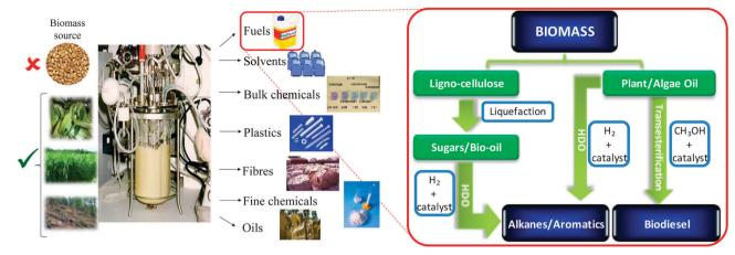
Scheme 2 Biorefinery routes for the co-production of chemicals and transportation fuels from biomass.
