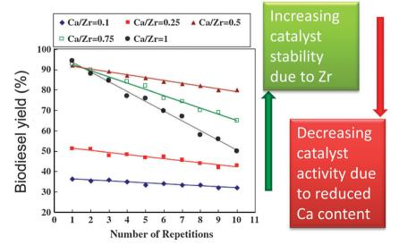
Fig. 4 Effect of Zr-doping on CaO solid base catalysts for biodiesel production. Adapted from reference 112. Copyright (2012), with permission from Elsevier
