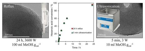
Fig. 9 Surfactant template extraction via energy/atom efficient ultrasonication delivers a one-pot PrSO<sub>3</sub>H-SBA-15 solid acid catalyst with identical structure and reactivity to that obtained by conventional, inefficient reflux. Adapted from ref. 172 with permission from The Royal Society of Chemistry.
