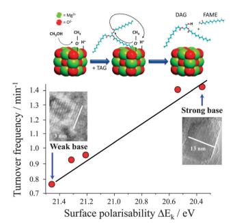
**Fig. 1** Relationship between surface polarisability of MgO nanocrystals and their turnover frequency towards tributyrin transesterification. Adapted from ref. 90 with permission from The Royal Society of Chemistry.
