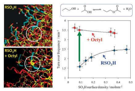
Fig. 16 (left) Molecular dynamics simulations of MCM-SO<sub>x</sub>H and MCM-Oc-SO<sub>x</sub>H pore models highlighting the interaction between surface sulfonic acid and hydroxyl groups in the absence of co-grafted octyl chains; (right) influence of PrSO<sub>3</sub>H surface density and co-grafted octyl groups on catalytic performance in acetic acid esterification with butanol. Adapted from ref. 213 with permission from The Royal Society of Chemistry.
