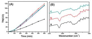
Fig. 2 (A) Plots of CO formation *versus* time in the absence (- ■ -) and presence of 1.5 M 2,2,2-trifluoroethanol (- • -), 3% (v/v) H<sub>2</sub>O (- • -), and 10% (v/v) H<sub>2</sub>O (- ▼ -) for 10 mg **ReC** (0.1 μmol)/H-TiO<sub>2</sub>/Dye (1.5 μmol) in 3 mL DMF containing 0.1 M SD; irradiation at > 420 nm. (B) IR spectra of **ReC**/H-TiO<sub>2</sub>/Dye in KBr discs (sample: KBr  $\approx 1:100$ ) before (a) and after irradiation for 100 min (b) and for 20 h (c).
