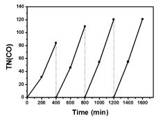
Fig. 3 Formation of CO in a 4-cycle repetition of irradiation at > 420 nm for 400 min after CO $_2$  bubbling for 30 min in the dark; 10 mg Dye/S-TiO $_2$ / ReC with 0.1  $\mu$ mol ReC and 1.5  $\mu$ mol Dye in the presence of 0.1 M SD and 10% (v/v) H $_2$ O.
