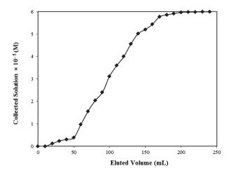
Fig. 10 Breakthrough curve for Rose Bengal-bottom ash column.
