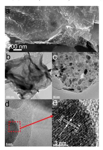
Fig. 3 (a) SEM, (b) and (c) TEM, (d) HRTEM images of M1-GNS, and (e) enlarged HRTEM image of the selected area marked by a box in (d).
