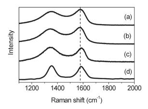
**Fig. 6** Raman spectra of (a) GNS, (b) M2-GNS, (c) M1-GNS, and (d) graphene sheets obtained from M1-GNS after removing the Fe<sub>3</sub>O<sub>4</sub> nanoparticles.
