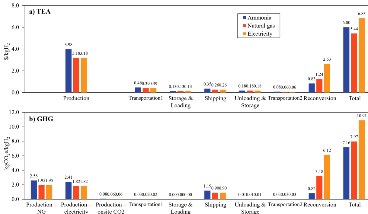
Fig. 7 Effects of reconversion fuel option on (a) LCOH and (b) GHG emission (U.S. to Japan, ATR-CCS-OC, grid electricity use, MDO for shipping fuel, 17.2 tonnes H 2 per h delivery).
