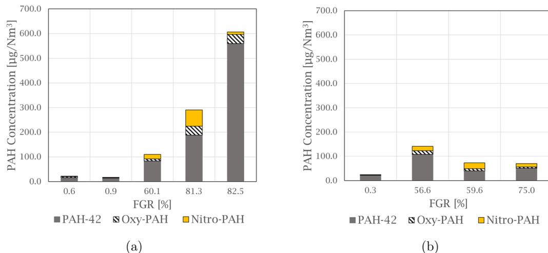
Fig. 1 Graphs showing the total PAH-42, oxy- and nitro-PAH concentrations in the off-gas at varying FGR levels for experiments at (a)  $1000 \text{ Nm}^3 \text{ h}^{-1}$  and (b)  $500 \text{ Nm}^3 \text{ h}^{-1}$ .
