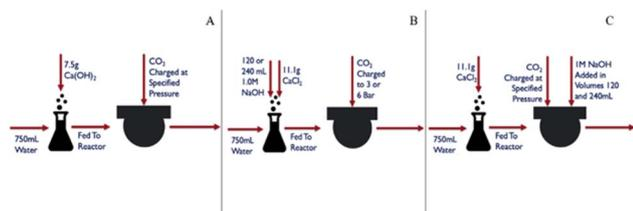
Fig. 2 Experimental reaction pathways: (A) pressure variation experiments of calcium hydroxide carbonation; (B) *ex situ* base addition carbonation of calcium chloride solution; and (C) *in situ* base addition carbonation of calcium chloride solutions.
