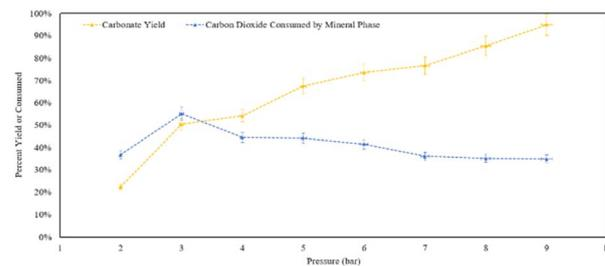
**Fig. 15** Percent yield of the residues and percent of CO<sub>2</sub> mineralized from what was provided to the reaction in the pressure varied calcite formation trials.
