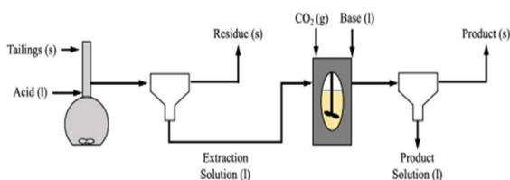
Fig. 1 Process flow diagram for pH swing process.
