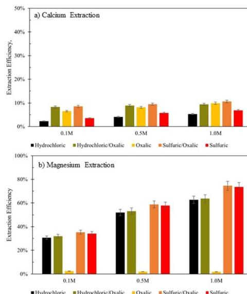
Fig. 12 Extraction efficiency of (a)  $\text{Ca}^{2+}$  and (b)  $\text{Mg}^{2+}$  in mineral acid series dissolution, compared to single acid dissolution. Data organized by the solution concentration step of the series. Naming convention refers to the order of the acid(s) used.
