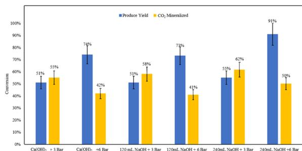
Fig. 18 Measured product yields and CO<sub>2</sub> mineralization quantities based on mineral carbonation experiments.
