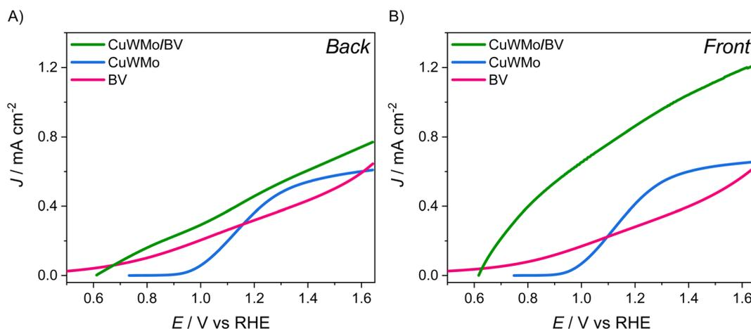
Fig. 7 Linear sweep voltammetry (LSV) scans recorded with CuWMo (blue), BV (magenta) and CuWMo/BV electrode (green) under (A) back-side and (B) front-side irradiation.
