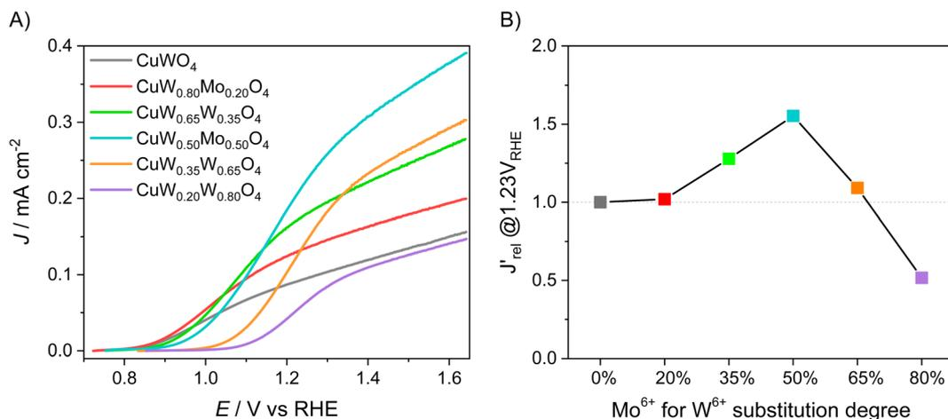
Fig. 2 (A) Linear sweep voltammetry (LSV) scans of  $\text{CuW}_{1-x}\text{Mo}_x\text{O}_4$  films with different  $\text{Mo}^{6+}$  for  $\text{W}^{6+}$  substitution degrees, under back-side irradiation. (B) Trend of the relative photocurrent efficiency  $J_{\text{rel}}^{\prime}$ , defined in the main text, vs. the percent of Mo for W substitution degree.
