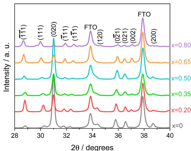
Fig. 1 XRD patterns in the 28° to 40° 2θ region of CuW<sub>1-x</sub>Mo<sub>x</sub>O<sub>4</sub> electrodes, with x = 0–0.8. The characteristic Miller indices of pure CuWO<sub>4</sub> wolframite single crystal structure (JCPDF 72-0616)<sup>34</sup> are indicated. FTO peaks are also reported.
