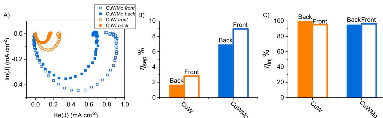
Fig. 6 (A) IMPS analyses at 1.6  $V_{RHE}$  for CuWMo (blue) and CuW (orange) electrodes in 0.1 M  $\text{K}_3\text{BO}_3$  under back- (full symbols) and front-side (void symbols) irradiation. The represented raw data were obtained upon normalization to the electron current recorded using the IMPS setup. (B) Charge separation ( $\eta_{sep}$ ) and (C) charge injection ( $\eta_{inj}$ ) efficiencies calculated from IMPS data under back- (filled columns) and front-side (void columns) irradiation.
