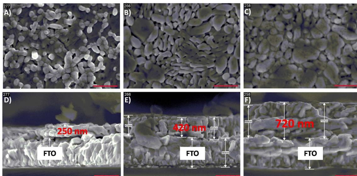
Fig. 3 (A–C) Top view and (D–F) cross section SEM images at 50 $\times$  magnification of (A and D)  $\text{CuW}_{0.5}\text{Mo}_{0.5}\text{O}_4$  1L, (B and E)  $\text{CuW}_{0.5}\text{Mo}_{0.5}\text{O}_4$  2L and (C and F)  $\text{CuW}_{0.5}\text{Mo}_{0.5}\text{O}_4$  3L films. The scale bar is 500 nm.
