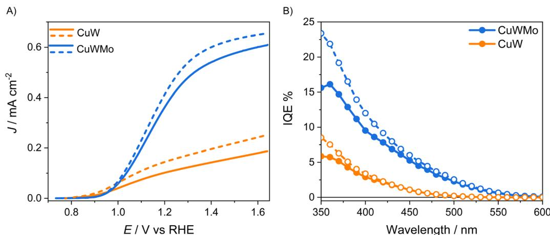
**Fig. 4** (A) Linear sweep voltammetry (LSV) and (B) internal quantum efficiency (IQE) curves at 1.23  $V_{\text{RHE}}$  of the CuWMo (blue) and CuW (orange lines) electrodes with comparable film thickness, in 0.1 M  $\text{K}_3\text{BO}_3$ , under back- (solid lines, full circles) and front-side irradiation (dashed lines, void circles).
