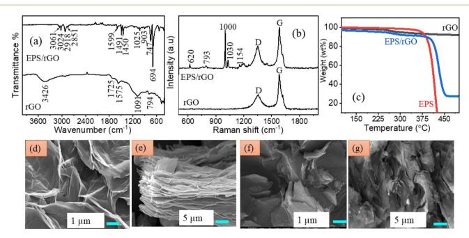
Fig. 2 (a) FT-IR (b) Raman spectrum of pure rGO and EPS/rGO composite (c) TGA curves of rGO, EPS, EPS/rGO (d, e) FE-SEM images pure rGO (f, g) FE-SEM images of EPS/rGO composite.
