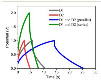
Fig. 8 GCD curves recorded for two different symmetric coin cell supercapacitor devices (D1 and D2) connected in parallel and series at a current density of 1 mA cm<sup>-2</sup>.
