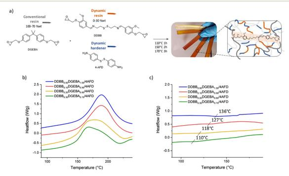
Fig. 6 (a) Synthesis of DDBB<sub>x</sub>DGEBA<sub>v</sub>/4AFD-based epoxy vitrimers (b) DSC thermograms obtained at a heating rate of 10 °C min<sup>-1</sup> for  $DDBB_xDGEBA_v/4AFD$  mixtures (c) corresponding  $T_q$  obtained during a second heating ramp at 10 °C min<sup>-1</sup>.
