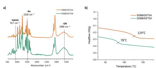
Fig. 4 (a) FTIR spectra of SDBB (orange) and DDBB (green) after curing (b) DSC thermograms of SDBB and DDBB after curing.
