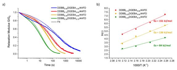
Fig. 7 (a) Stress relaxation experiments at 190 °C of DDBB<sub>x</sub>DGEBA<sub>v</sub>/4AFD formulations with x ranging from 0 to 0.30 and y from 1.00 to 0.70 and (b) corresponding Arrhenius dependence.
