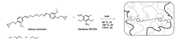
Fig. 3 Synthesis of epoxy SDBB/DETDA and DDBB/DETDA-based vitrimers.
