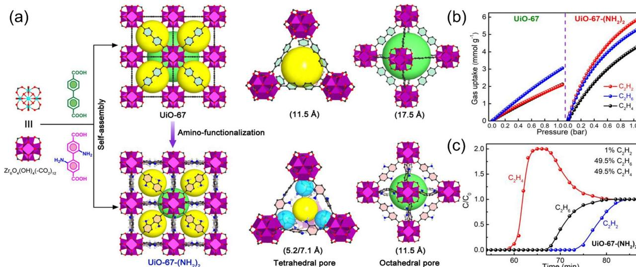
Fig. 6 (a) Comparison of the crystal structures, tetrahedral cages, and octahedral cages of UiO-67 and UiO-67-( $\text{NH}_2$ )<sub>2</sub>. (b) Gas adsorption isotherms of UiO-67 (left) and UiO-67-( $\text{NH}_2$ )<sub>2</sub> (right) at 296 K. (c) Experimental column breakthrough curves of UiO-67-( $\text{NH}_2$ )<sub>2</sub> for 1/49.5/49.5 ternary mixtures under ambient conditions. Reproduced with permission from ref. 36. Copyright © 2022, American Chemical Society.
