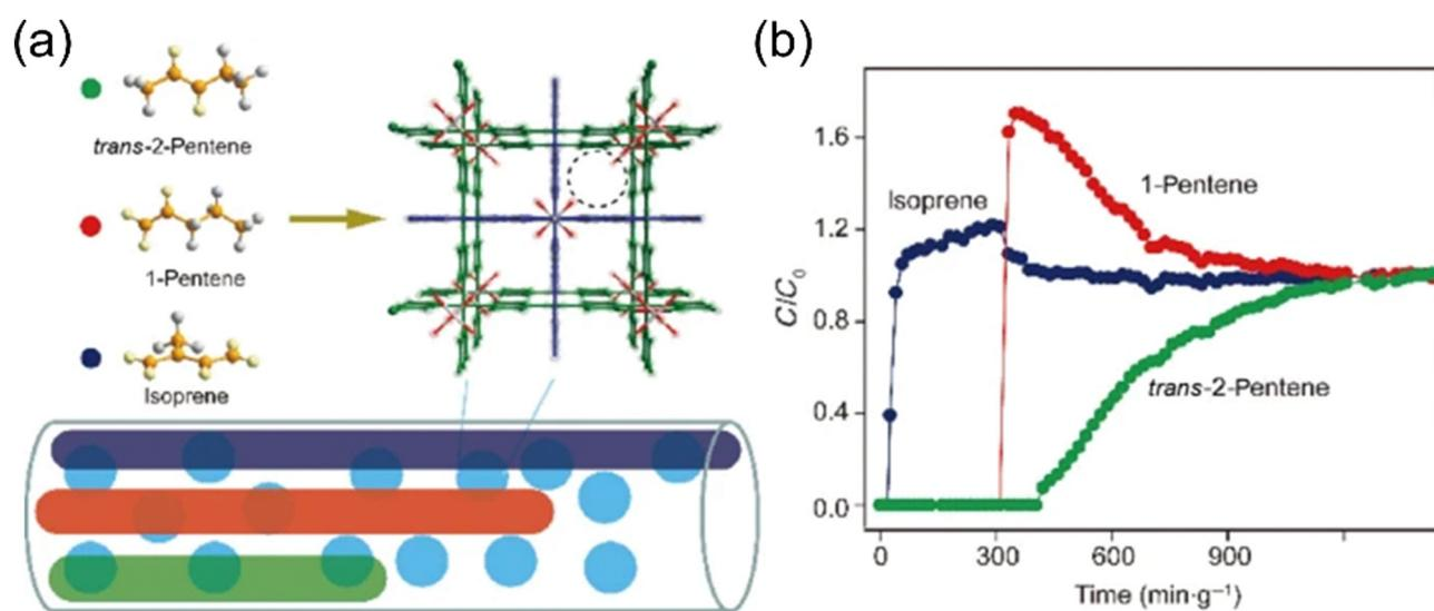
Fig. 12 (a) Schematic diagram of TIFSIX-2-Cu-i and ZU-62 for the separation of *trans*-2-pentene/1-pentene/isoprene. (b) The breakthrough performance of TIFSIX-2-Cu-i for *trans*-2-pentene/1-pentene/isoprene/ $\text{N}_2$  (9%/9%/9%/73%, v/v/v/v) ternary mixtures. Reproduced with permission from ref. 94. Copyright © 2021, Springer Nature Publishing AG.
