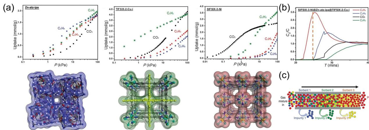
Fig. 9 (a) Structure and adsorption isotherms of three high-performance ultra-porous MOFs. (b) One step separation of high purity  $C_2H_4$  in a four-component hybrid system. (c) Diagram of the synergy of the three MOFs. Reproduced with permission from ref. 4. Copyright © 2019, The American Association for the Advancement of Science.
