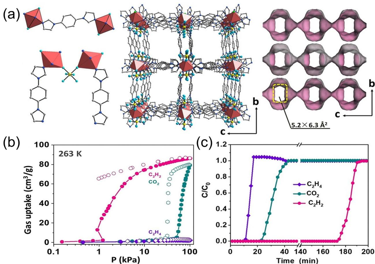
Fig. 7 (a) Structure and channel of NTU-65. (b) C<sub>2</sub>H<sub>2</sub>, C<sub>2</sub>H<sub>4</sub>, and CO<sub>2</sub> adsorption isotherms of NTU-65 at 263 K. (c) Breakthrough curves of NTU-65 at 263 K. Reproduced with permission from ref. 65. Copyright © 2020, Wiley-VCH GmbH.
