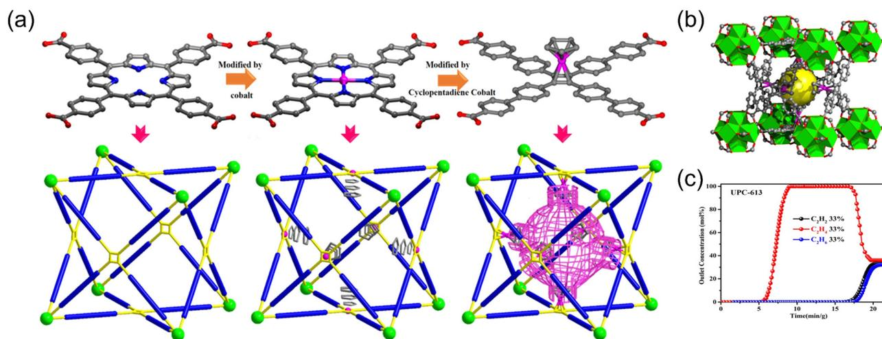
Fig. 4 (a) The progressive process of linker modification based on ftw topology platform in Zr-MOFs. (b) Three-dimensional view of unit cubic cages. (c) Experimental column breakthrough curves for  $C_2H_6/C_2H_4/C_2H_2$  (33/33/33) mixtures absorber bed packed with UPC-613. Reproduced with permission from ref. 50. Copyright © 2020, Wiley-VCH GmbH.
