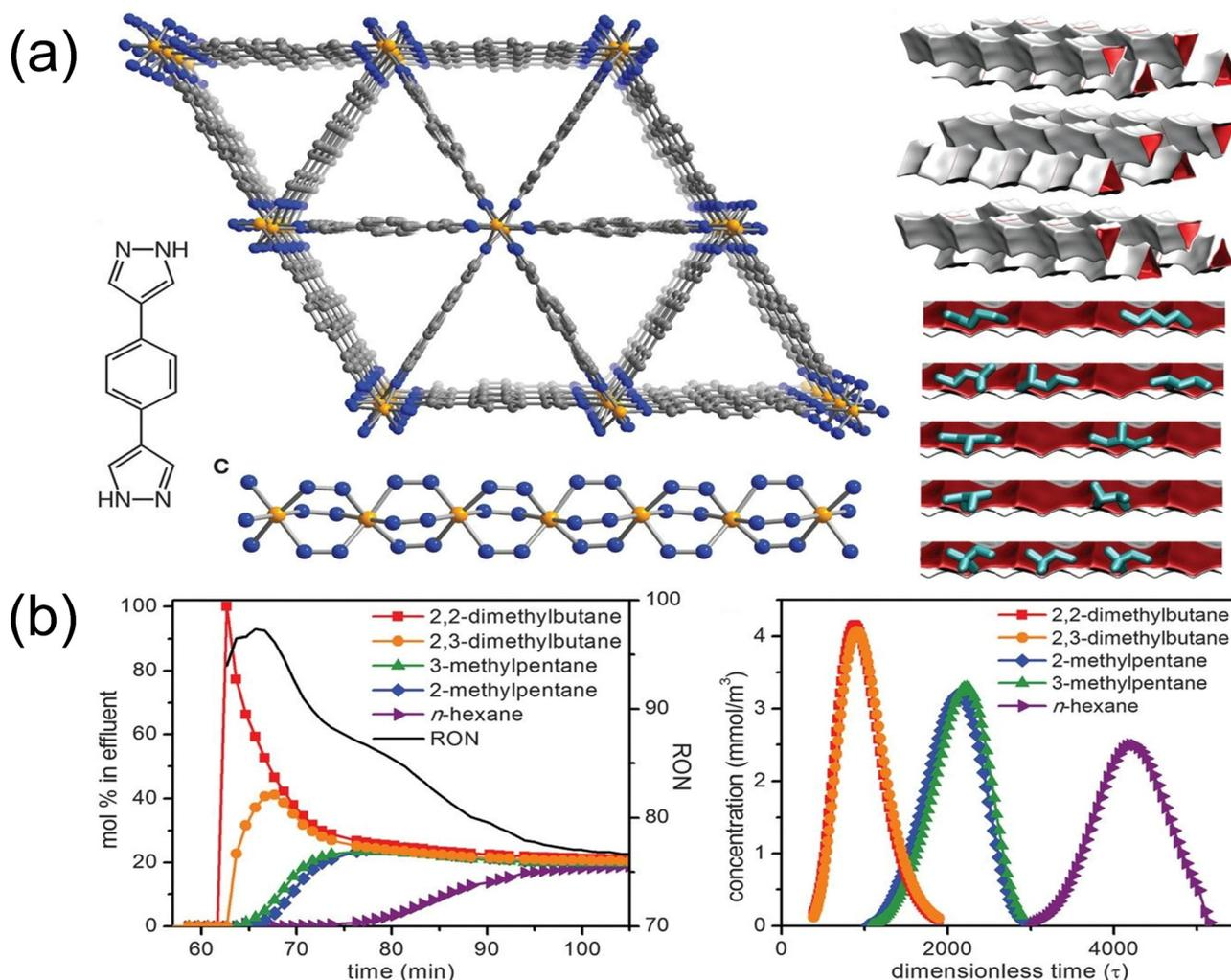
Fig. 13 (a) Structures of  $\text{Fe}_2(\text{bdp})_3$ . (b) Mixture breakthrough curves of an equimolar mixture of 2,2-dimethylbutane, 2,3-dimethylbutane, 3-methylpentane, 2-methylpentane, and *n*-hexane running through a packed bed of  $\text{Fe}_2(\text{bdp})_3$  at 160 °C. Reproduced with permission from ref. 96. Copyright © 2013, The American Association for the Advancement of Science.
