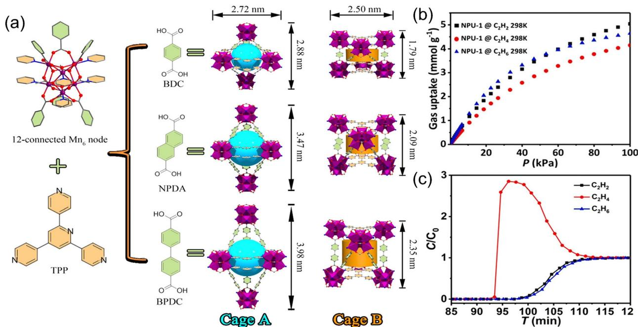
Fig. 3 (a) A series of isostructural MOFs (NPU-1/2/3) with double caged cavities. (b)  $C_2$  gas sorption isotherms of NPU-1. (c) Experimental breakthrough curves of  $C_2H_2/C_2H_4/C_2H_6$  separation (1:1:1) based on NPU-1 at 298 K. Reproduced with permission from ref. 49. Copyright © 2021, American Chemical Society.
