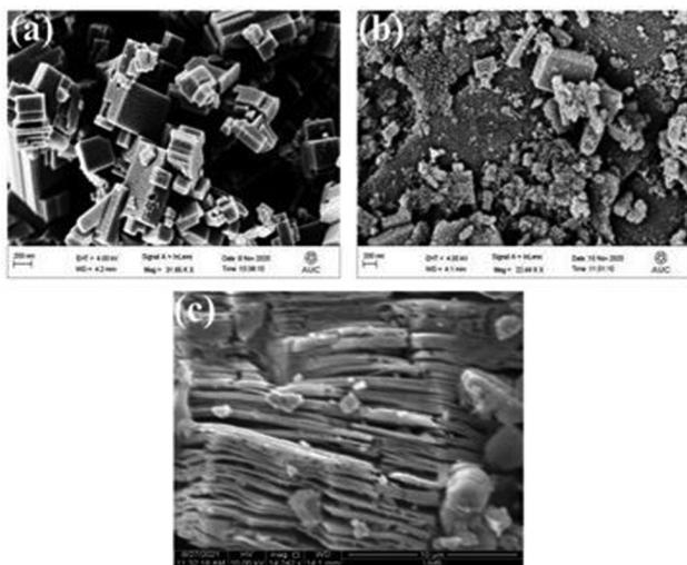
Fig. 5 SEM images of (a)  $\text{WO}_3$ , (b)  $\text{WO}_3$ -MXene, and (c) MXene. Reproduced from ref. 80 with permission from MDPI, copyright 2022 under a Creative Commons Attribution 4.0 International License (CC BY 4.0).
